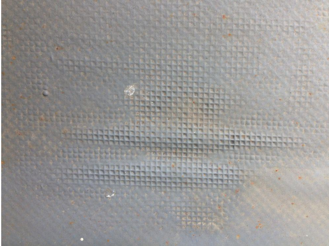
Figure 10. Close up, Material 1.2mm, Age approx. 4 years.
