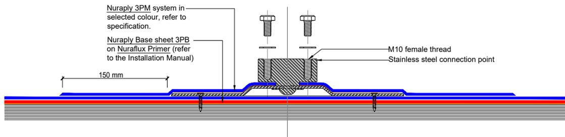
SECTIONAL ELEVATION: CENTRE FIXING NOT SHOWN
