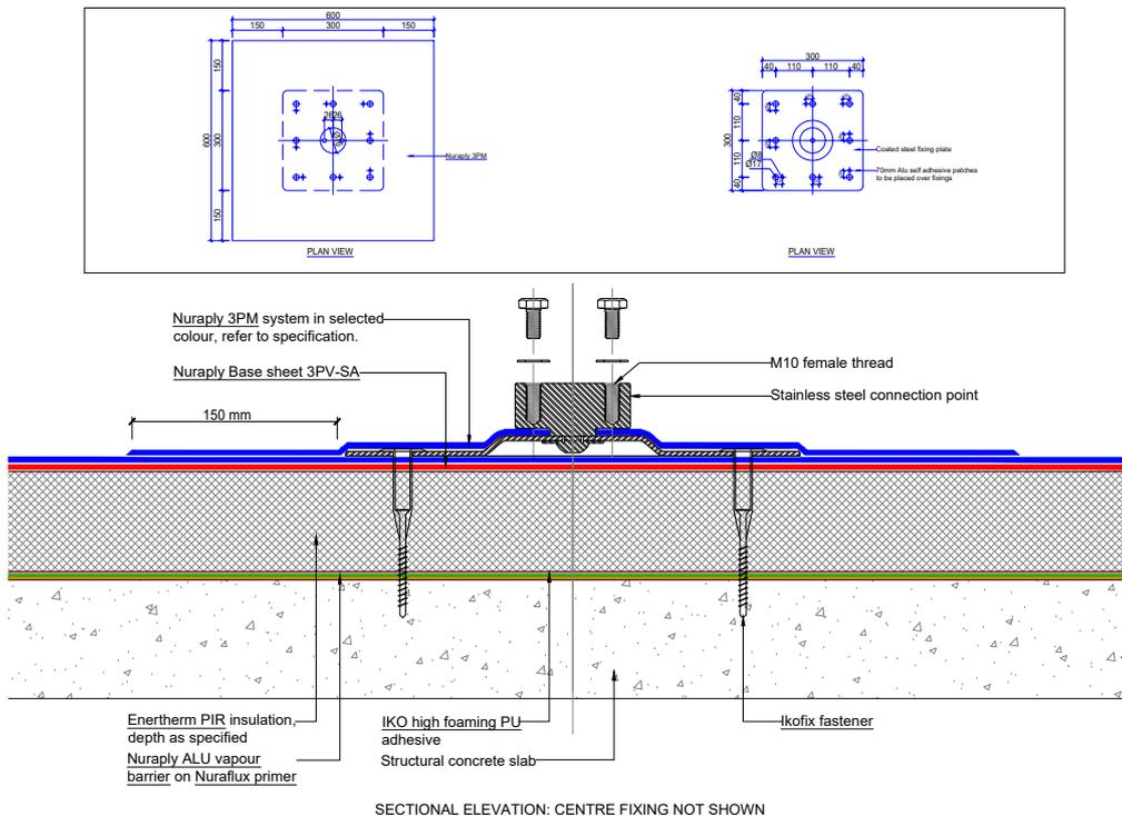
SECTIONAL ELEVATION: CENTRE FIXING NOT SHOWN
