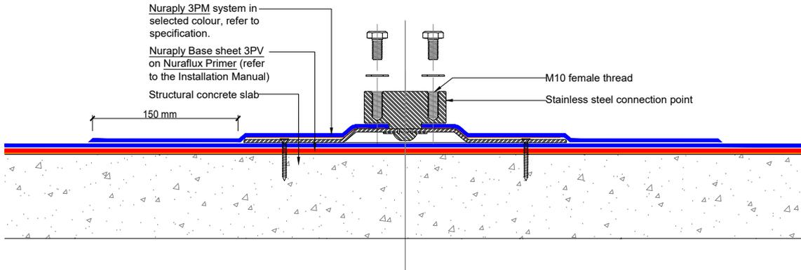
SECTIONAL ELEVATION: CENTRE FIXING NOT SHOWN
