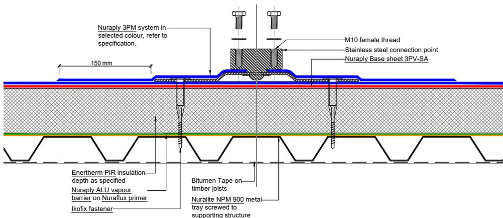
SECTIONAL ELEVATION: CENTRE FIXING NOT SHOWN
